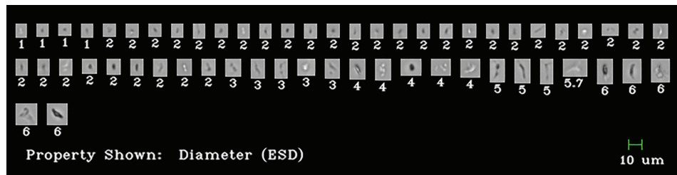
Figure 4 – NIST Protein Reference Standards as imaged with a standard 10 \times air objective flow imaging system. (Particle size shown below each image in microns ranging from 1–6 \mu\text{m} .)
