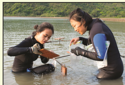
Deploying settlement plates as part of a monitoring program in Yueng Shui O, Hong Kong. Credit: Lori Cheung
