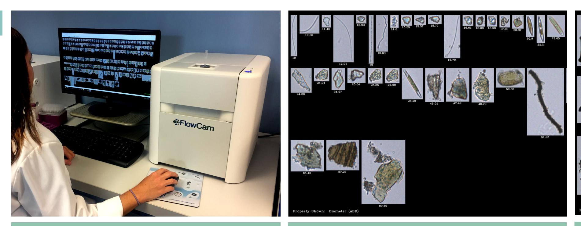
**Figure 1.** The FlowCam is a particle analyzer that is effective at analyzing microplastics using its imaging and analysis capabilities. Credit: Fluid Imaging Technologies, Inc.
