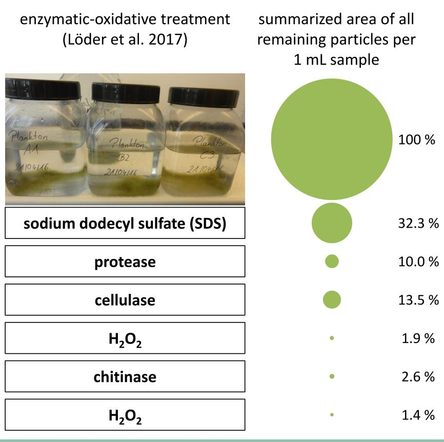
**Figure 7.** (Above) The six-step digestion used by Lorenz et al. to isolate microplastics from organic matter in marine water samples. Each step shows a reduction in area of remaining particulate matter, as calcuated by VisualSpreadsheet using FlowCam images. Credit: Lorenz et al. (2017).
