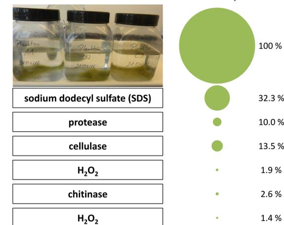
**Figure 7.** (Above) The six-step digestion used by Lorenz et al. to isolate microplastics from organic matter in marine water samples. Each step shows a reduction in area of remaining particulate matter, as calculated by VisualSpreadsheet using FlowCam images. Credit: Lorenz et al. (2017).
