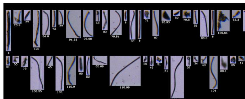
**Figure 4.** (Above) Polyethylene terephthalate microplastic fibers (MPF) as imaged by the FlowCam. The crisp, non-weathered edges of the above MPF distinguished these from other naturally-occurring, weathered fibers. Credit: Woods et al. (2017).
