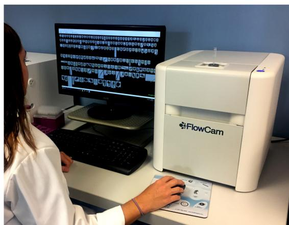
**Figure 1.** The FlowCam is a particle analyzer that is effective at analyzing microplastics using its imaging and analysis capabilities. Credit: Fluid Imaging Technologies, Inc.
