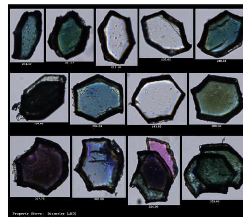
**Figure 3.** Multi-colored plastic glitter as imaged by the FlowCam at 4X. Credit: Fluid Imaging Technologies, Inc.
