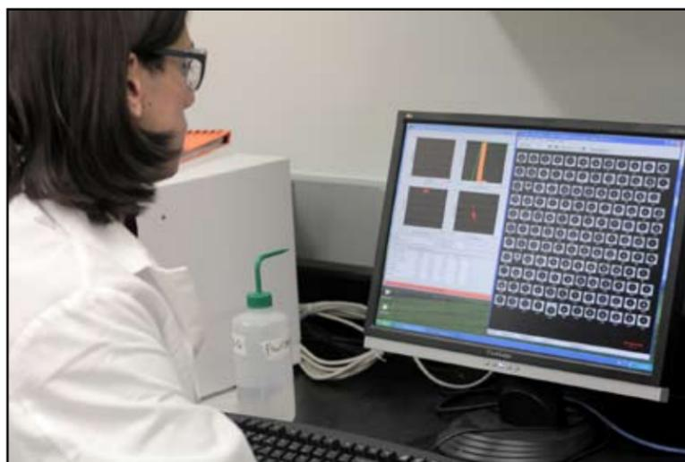
air bubbles, as opposed to counts and graphs offered by other systems. It also could detect opaque, translucent, and transparent particles and automatically discern one from the other using pattern recognition software. The FlowCAM could also determine why the particles were present and whether the particles detected were related to the product formulation or to sampling technique.
