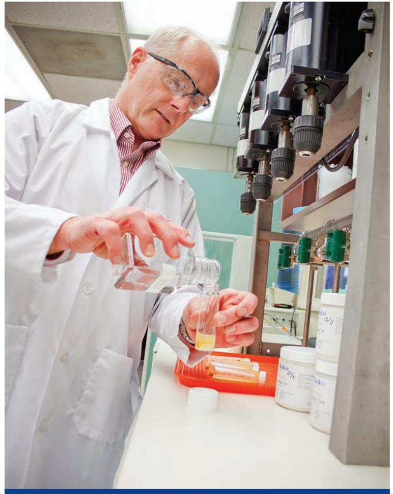
**Ross Clark** prepares a dry product sample for testing on the FlowCAM. The imaging particle analysis instrumentation automatically takes high resolution, digital images of individual particles and measures each one using up to 32 different parameters in real time. "The FlowCAM is the only instrumentation on the market that bases its measurements on the actual size and shape of the particle," says Clark.
