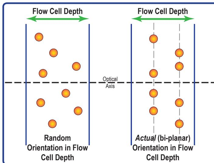
Figure 2: Side-view of flow cell depth dimension along the optical axis, showing random particle distribution through the depth on left, and actual bi-planar distribution on right.
