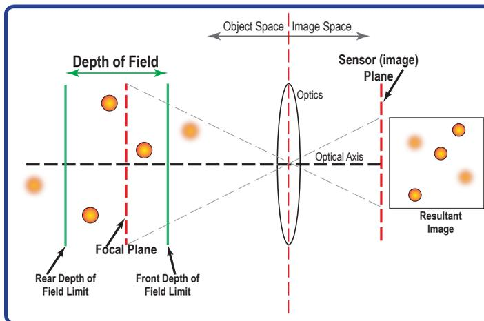
Figure 1: Side-view diagram showing focal plane, image plane and depth of focus for a simple optical system. To the right of the sensor plane is a depiction of the resultant image.
