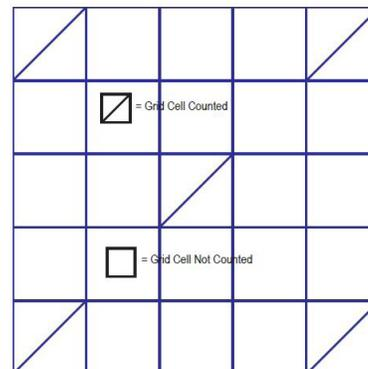
Because of the time involved for an operator to do manual counting, only a small number of actual grid cells are counted, with the results then being interpolated as an average number. Not only is the sample size very small, which yields low statistical significance, but it is known that up to 25% error can be introduced merely by "operator interpretation".
