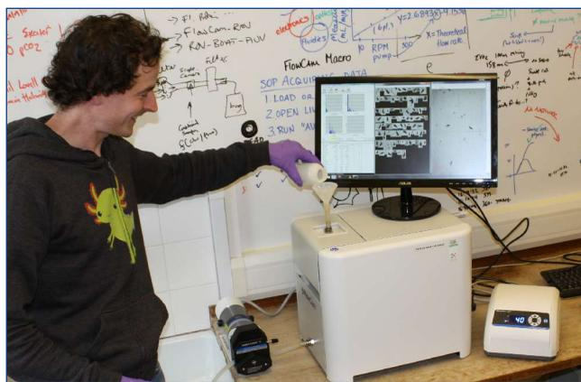
(Top) A laboratory technician operates the FlowCam Macro installed at the SAHFOS laboratory in Plymouth, England. (Bottom) Observations of particles from a conventional continuous plankton recorder (CPR) sample obtained with the FlowCam Macro. Images are shown of plankton (left panel), descriptive statistics (central panel), and images grouped into classification types (right panel).
